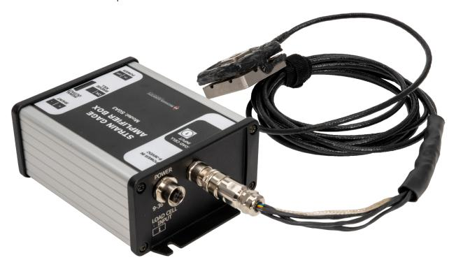
Connect power input cable to the back of the Multi-Channel Strain Gage Amplifier.
