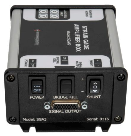
Turn on power to amplifier box. The load cells should now output a voltage proportional to experienced forces. The sensitivities for each load cell can be found on their associated calibration sheet. Each signal has a  $\pm$  10 V measurement range. Transducer unbalance (no-load output) should be removed in the data-acquisition system through either nulling the channels before recording or during post-processing.
